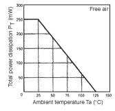
In case the total dissipation exceeds the permissible power dissipation, either attach a radiator plate to the transistor, or replace the transistor.
