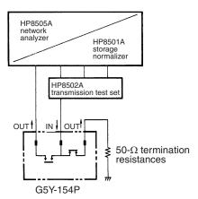
The following characteristics are measured with contacts unrelated to the measurement terminated at  $50\Omega$ , when a signal is applied from input terminal 11 to output terminal 8 or from input terminal 11 to output terminal 14 of the sample.
