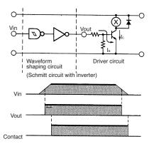
If the Schmitt trigger circuit is configured of transistors, a residual voltage may exist in the output of the circuit. Therefore, confirm that the rated voltage is present across the relay coil, or that the residual voltage drops to zero when the relay releases.
