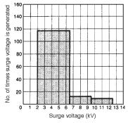
Note: This graph is plotted by measuring the surge voltage in the line of low-tension overhead wiring (cable length: 200 to 500 m).
