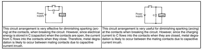
Although it is considered that switching a DC inductive load is more difficult than a resistive load, an appropriate contact protection circuit can achieve almost the same characteristics.
