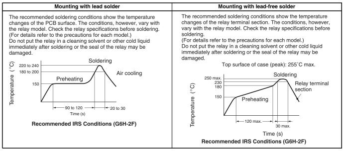
Note: Do not submerse the relay in a solder bath. Doing so will deform the resin, causing faulty operation.
