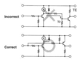
A circuit that produces a control output as soon as the relay operates must be carefully designed. In the first example, electrode dark current flows as shown when the relay operates. When dark current flows into the relay coil, the relay's resistivity to shock and vibration may degrade.
